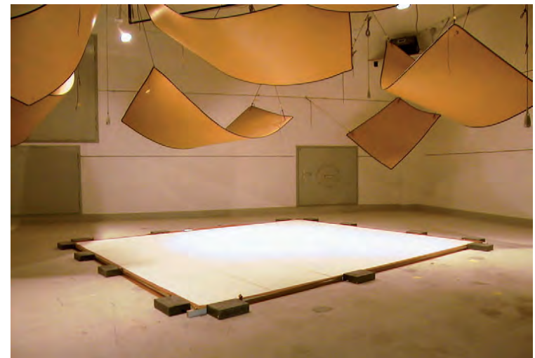
Random Incidence Sound Absorption in a Reverberation Room
